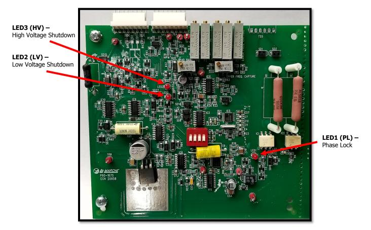
Figure 6 – S2A-167S Oscillator/Line Sync Board
