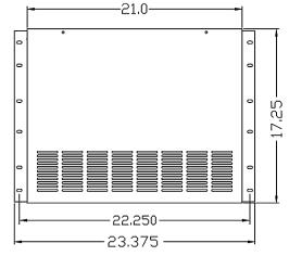
Figure 3 – 9D/9E Enclosure Bolt Pattern
