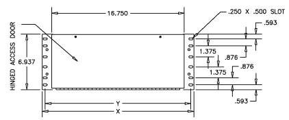
Figure 1 - 39 Enclosure Bolt Pattern
