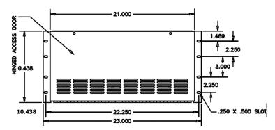
Figure 2 - 33 Enclosure Bolt Pattern
