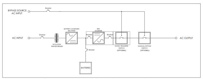
**Figure 5** – One-Line Diagram for Typical A31 Inverter Application
