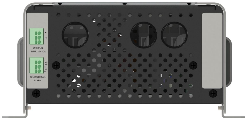
Figure 7 - Charger Alarm Connections
