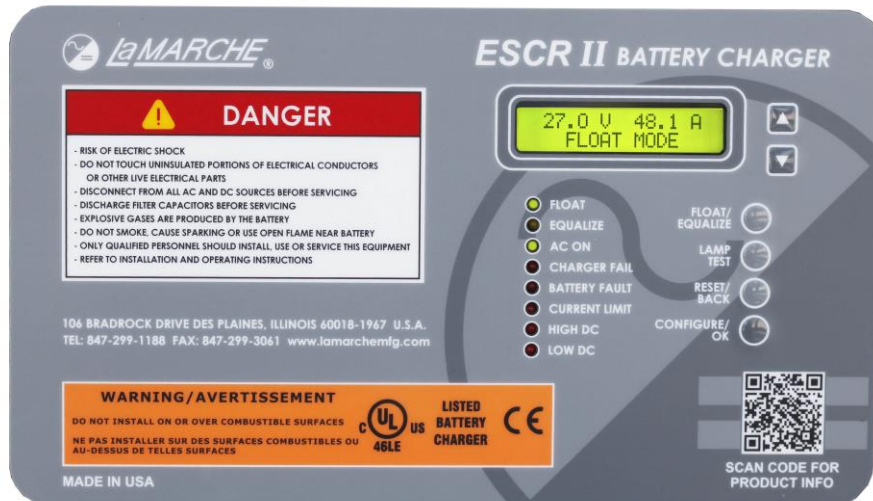
Figure 6 - Front Panel Display (Unit in Float Mode)
