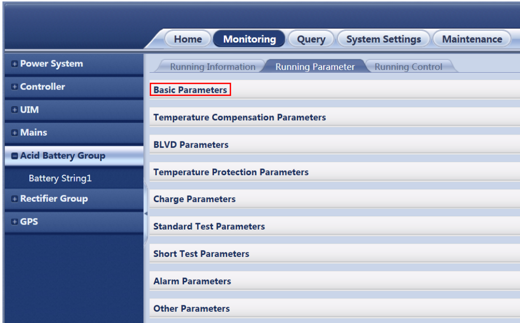
Figure 8-10 Setting basic battery parameters on the WebUI
