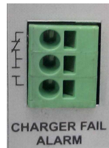
Figure 4 Charger Fail Connections
